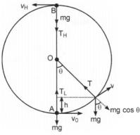
The forces acting on the body, when the string makes an angle  $\theta$  with the initial position are shown in the figure. Here, mg is the weight of body and T the tension in the string. If v be the instantaneous velocity at this point, then a centripetal force  $F = \frac{mv^2}{l}$  is required radially inward. From figure, it is clear that in equilibrium the centripetal force is provided by resultant of two forces i.e.,  $T - mg \cos \theta = \frac{mv^2}{l}$
