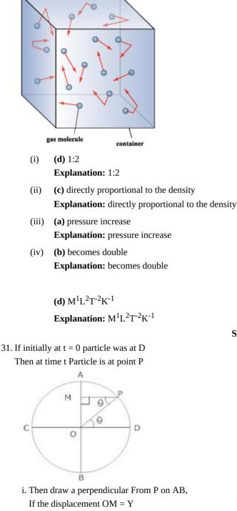
If the displacement OM = Y Ratios of circle of reference = Amplitude = a then In  $\triangle$ OMP,  $\angle$ POD =  $\angle$ OPM =  $\theta$  ( $\therefore$  Alternate Angles)  $sin\theta = \frac{OM}{OP}$
